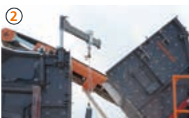
Blow-bar exchange system
