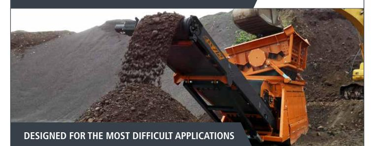
The RSS712 scalping screen is one of the most robust and reliable scalping screens on the market. Built to handle the toughest of applications, the RSS712 comes with a double deck vibrating screen and the longest stockpiling conveyor available.
