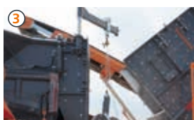
Blow-bar exchange system
